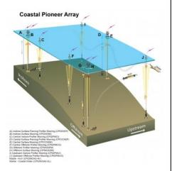
Figure 2. Schematic of the Coastal Pioneer Array of moored instrumented profilers. Our study used data from the profiler "G".
