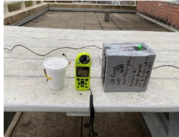
Figure 1.6- The TILTTING-23 Probe (far right) and a Windsond (far left) are used during the static test, observing temperature and relative humidity profiles outdoors and indoors.
