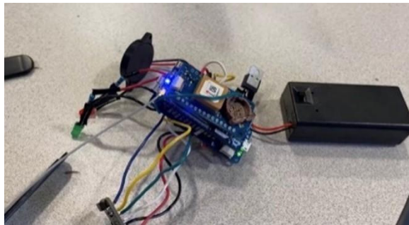
Figure 1.1 - The TILTTING-23 Probe in its wired construct before PCB development.
